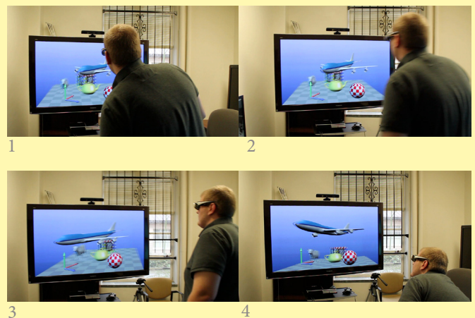
Images (above) show examples of the Kinect Virtual Reality research. The image on the display appears to be attached to the room rather than to the TV. As you move about, you perceive that you are moving around the displayed scene. The image becomes an extension of the room in which you stand, connected at the rectangular frame of the screen, rather than being a separate scene detached from reality by the display plane. This effect enhances the illusion that the displayed objects are 3D, solid, and separate from the display. Their presence and realness are astonishing.
